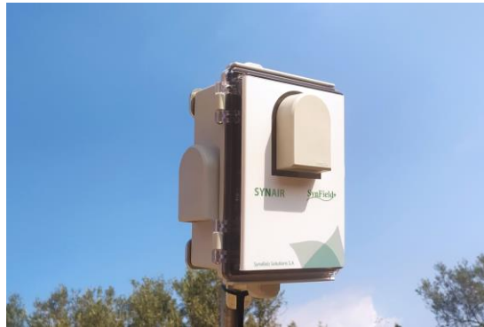
Figure 6: A SynAir™ Installation
